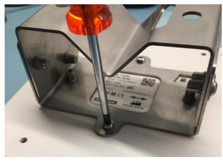
Optional MT40 tiltable pole mount needs to be attached to the TCR-S.
