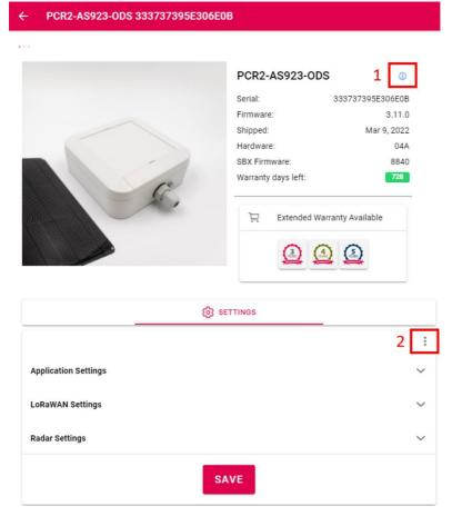
Start the PPX Configurator tool. After some seconds you will see the device information and settings.
