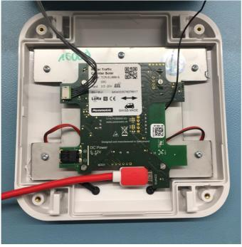
Connect the sensor to your Computer with a USB Cable using the Config Port.
