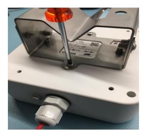
Optional MT40 tiltable pole mount needs to be attached to the PCR2-ODS.
