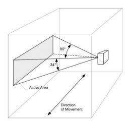
Installation height: Installation direction: Detection range: Separation angle: Avoid: 1.2...1.4m (4...5 feet) above floor
