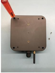
Remove the four screws from the casing to gain access to the device.
